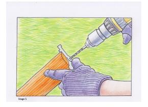
Locate the centre of the poles and drill a 13 mm (½ inch) diameter 60 mm deep hole (a 13 mm by 95mm auger bit when inserted into a chuck of a drill should provide the 13 mm drilling depth)
